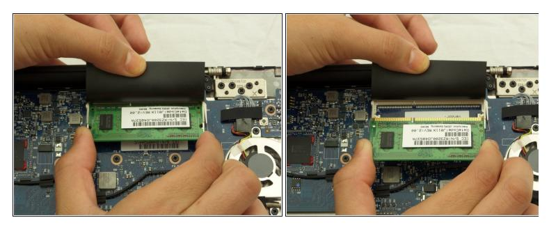
• Use two fingers to slide the RAM out at the angle that it has been released.
