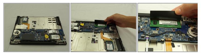
• Locate the RAM under a black flap alongside where the laptop screen and device body meet.
