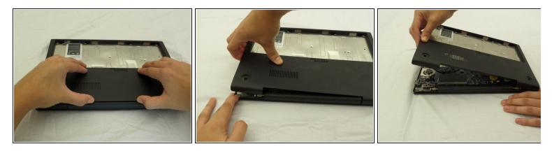
• Starting where the body of the laptop and the laptop screen meet, pry apart the lower case from the rest of the laptop.
