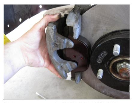
Place the caliper back on the rotor.
