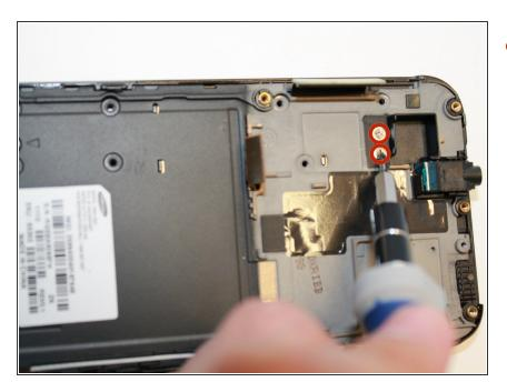
Remove screws with the #00 screwdriver.
