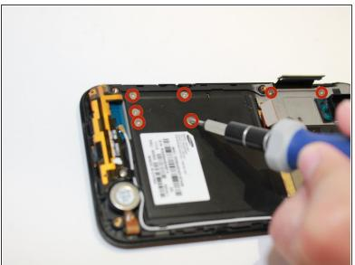
Remove the eight screws with the #00 screwdriver.
