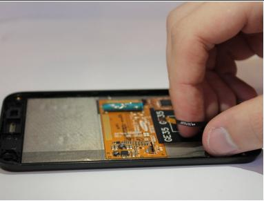
By using the plastic opening tool you can release the keypad flex cable from the jaw connecter clamp.
