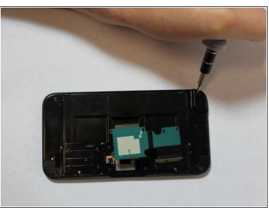
Remove the four corner screws using the #00 screwdriver.
