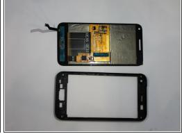
Using the plastic opening tool to pry around the edges, release the touch screen from the screen frame.
