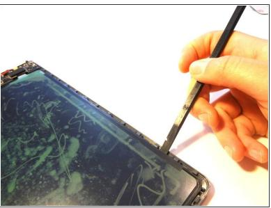
Use a spudger (or gently bend the back plate of the device) to unsnap the snaps holding the screen in place.
