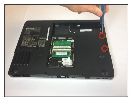
Remove the two 2.5mm Phillips #00 screws
