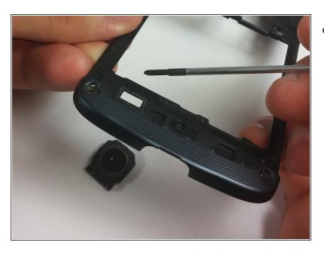
Insert your new speaker, in its enclosure, back onto the midframe.
