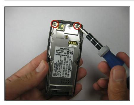
Remove the two screws at the top.
