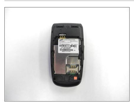
This is the back view following the removal of the back cover and battery.
