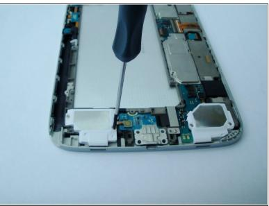
For each speaker remove the two 3-mm Phillips head screws using a Phillips #00 screwdriver.
