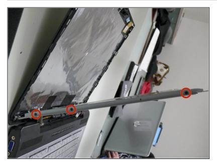
• Remove **3** Phillips 3.2 mm screws from each side of the metal case around screen.
