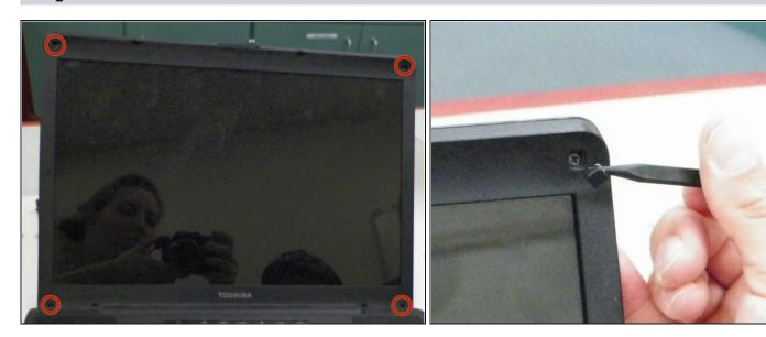
• Use <u>tweezers</u> to remove rubber screw covers on **4** corners of frame around screen.
