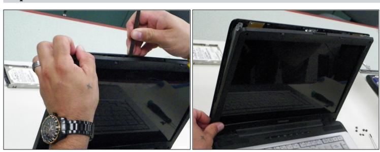
• Use flat side of spudger to pry the top and sides of the frame around screen.
