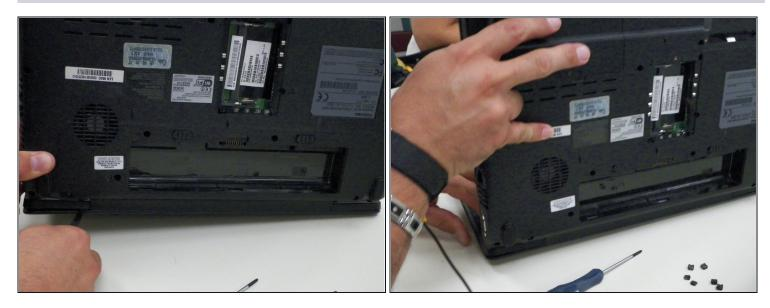
• Turn device onto its screen side to access the bottom of hinge portion of the screen and push bottom piece of frame along device hinge until it loosens.
