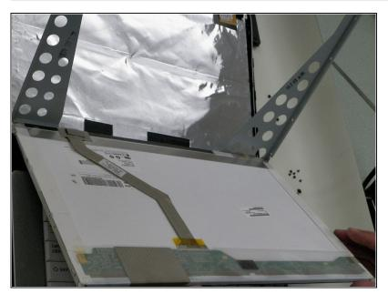
Pull the screen forward from the top out of the metal frame enough to see the back of the screen.
