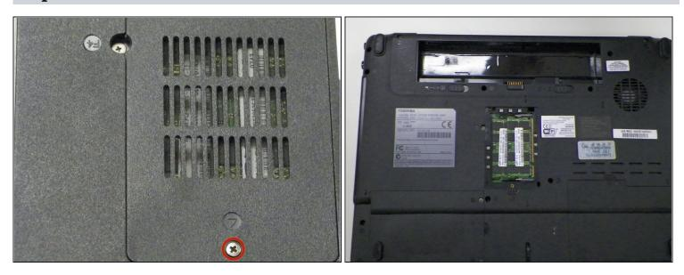
• Loosen **1** Phillips 4.2 mm size captive screw and lift cover off device to expose 2 RAM sticks.
