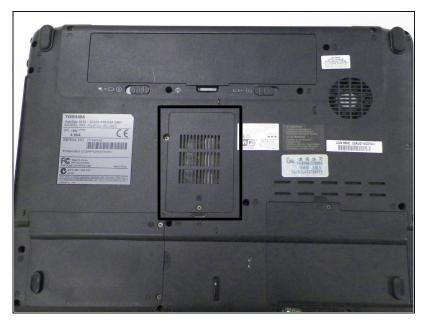
Locate the RAM vented plastic cover in the center of the device.
