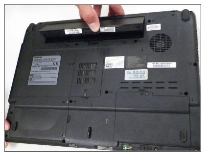
• Gently lift and pull the battery out of the device.
