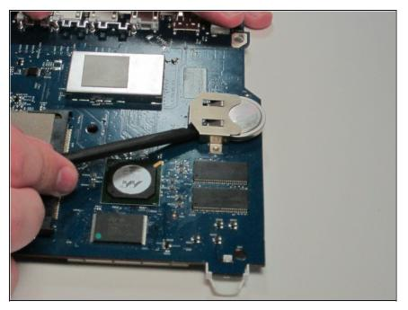
Gently slide out the battery with a small narrow tool such as a spudger. Insert a new 3V CR2450HR.
