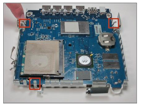
• Carefully push back the three metal tabs with your fingers on the sides of metal case.
