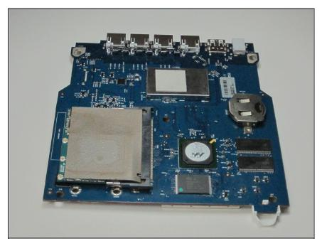
• Carefully pull the metal case away from the logic board.
