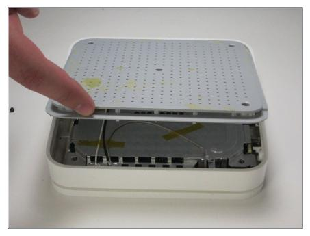
• Lift up the back case from the perforated edge to remove it.
