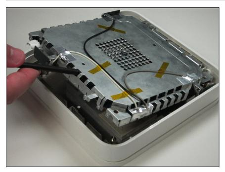
Remove logic board and metal casing from outer case by prying from one side using a spudger.
