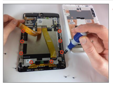
As shown, the battery is held in place by a total of 8 screws. Use the #00 Phillips screwdriver to remove all 8.
