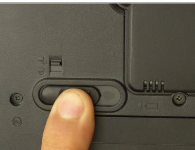
Use any finger to move the larger switch above the battery to the left and hold the switch.
