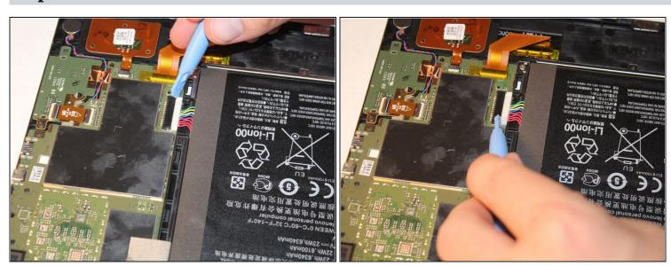
• Using either the plastic opening tool or your fingers, gently pull on both sides of the plug to release it.
