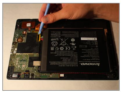
• Pull off the plastic that is covering the battery cable.
