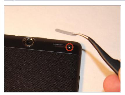
Remove the screws from both of the spots that were covered.
