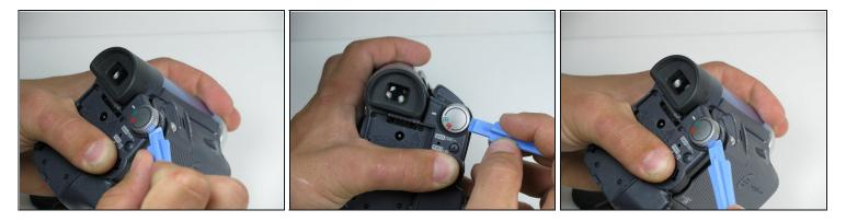
• Locate the blue plastic tool opener, then remove both the round record/playback and record/power control knobs by prying it open from the camcorder.
