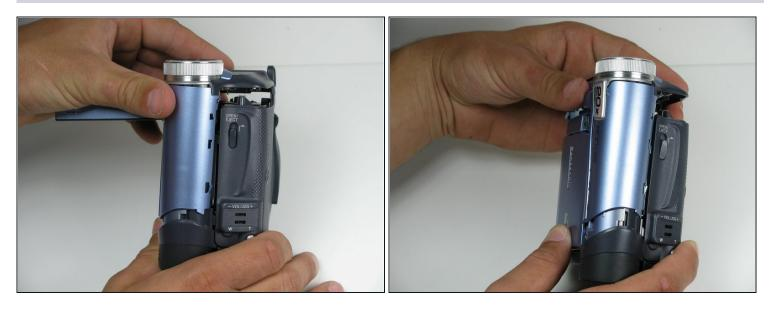
(*i*) Carefully remove the front cover from the body of the camcorder.
