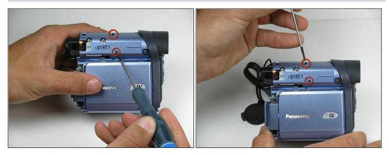
• Remove the indicated 4.5mm screws from the LCD side of the camera.
