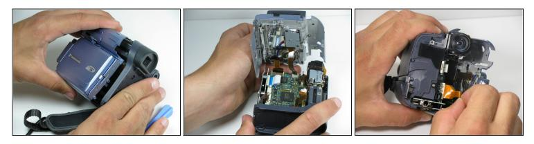
A Before removing the LCD panel from the camcorder, disconnect the ribbon cables joining the LCD panel to the logic board.
