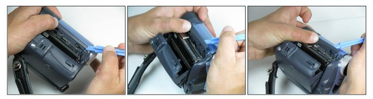
• Use the blue plastic opening tool to remove the gray trim piece by prying it from top of the camcorder.
