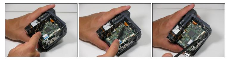
• Using the spudger, remove the few remaining ribbon cables from the logic board.
