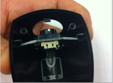
Insert your new board into the outer casing. Be sure that it rests firmly between the sets of rails on either side.
