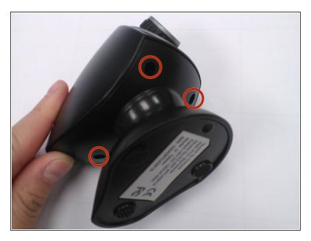
Using a Phillips-head screwdriver, remove each of the 3 screws from the underside of the camera head.
