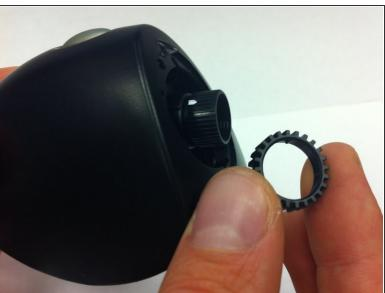
Remove the small, black, ridged inner ring around the lens with your fingers.
