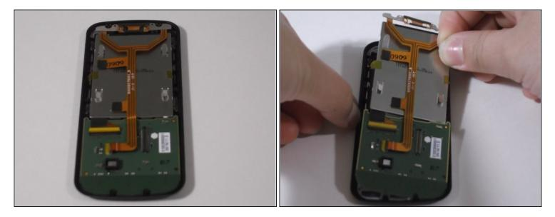
• Peel back the yellow tape on the side of the screen using tweezers or your fingernails. Lift away screen and board.
