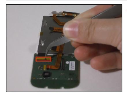
Pry the bar connecting the screen and circuit board by prying it gently upwards with tweezers to detach, separate, and remove the screen.
