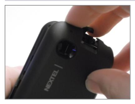
• Pull back until cover is removed. Place cover aside.
