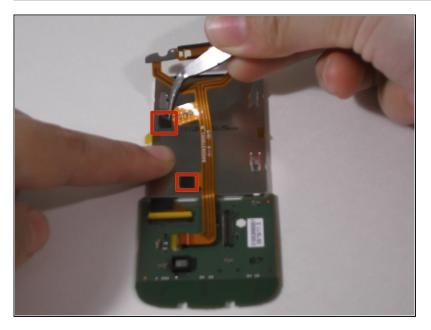
Lift the yellow strip away from the back of the screen by gently gripping with <u>tweezers</u> and detaching the two, black, square, contact points.
