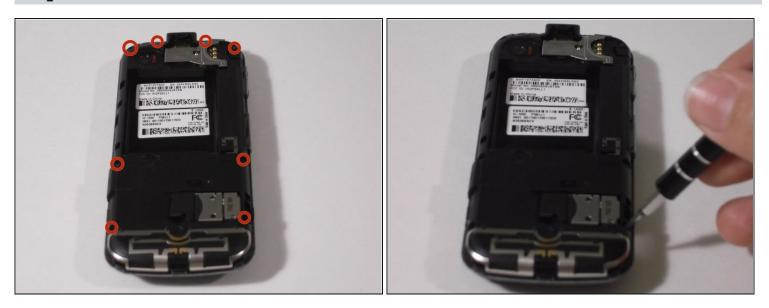
• Remove eight black .4 centimeter screws on the top, bottom, and sides of the phone with a T5 Torx screwdriver by inserting it into the screws and turning it to the left. Set screws aside.
