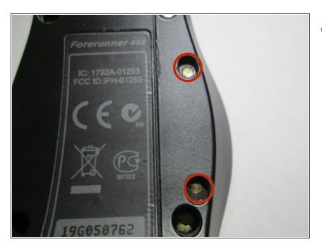
Locate corroded contacts on the back side of the watch.
