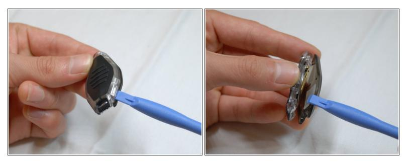
• Insert the plastic opening tool into the seam of the device.
