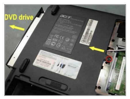
Locate the DVD drive and remove screw securing drive. Carefully push drive out from laptop.
