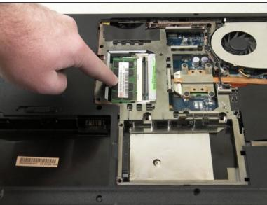
After removing screws, carefully detach cover. You will see the cooling fan in the corner.
