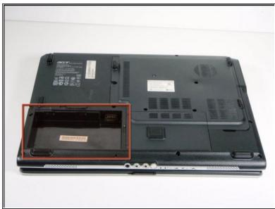
Locate tab with battery symbol on back of laptop. Slide to left to eject battery.
