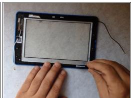
Again use a double side adhesive tape to install the the metal LCD frame.
