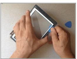
Use again hot air and a plastic tools to separate the metal screen frame / holder.
