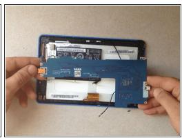
Unscrew 5x screws and rmove the main board.
