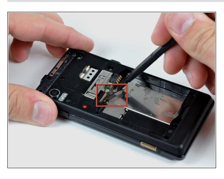
Insert the flat end of a spudger and pry downwards to release the plastic tab holding the rear case to the motherboard screw.
