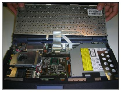
This picture is a top view of the computer after the speakers and keyboard have been removed.
