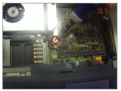
Locate the fan's screw and remove it using a small Phillips screwdriver.
