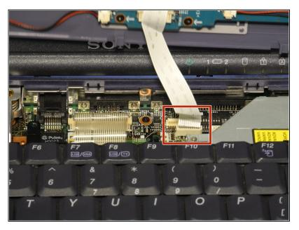
• Put the speaker panel's ribbon cable back in place.
