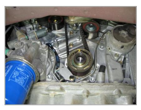
Lower cover removed (rubber plug in the dipstick opening to prevent trash from falling in)
