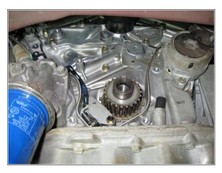
Bottom view showing the belt, pulleys, and tensioner removed
