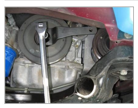
Crank pulley bolt removal (loosen the bolt before removing the motor mount!)
