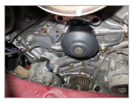
Top view showing water pump. Also showing the belt, pulleys, and tensioner removed
