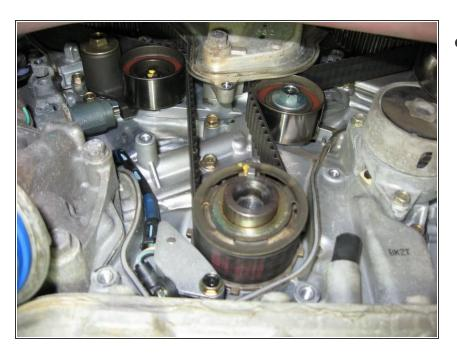
Different angle to show both 14mm pulley bolts
