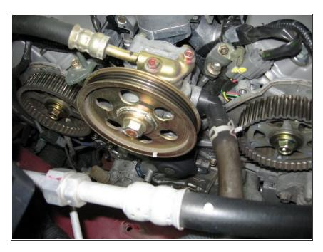
Top view showing timing belt, tensioner, and pulleys off
