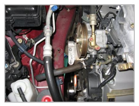
Looking from above showing the accessory belts removed along with the motor mount.
