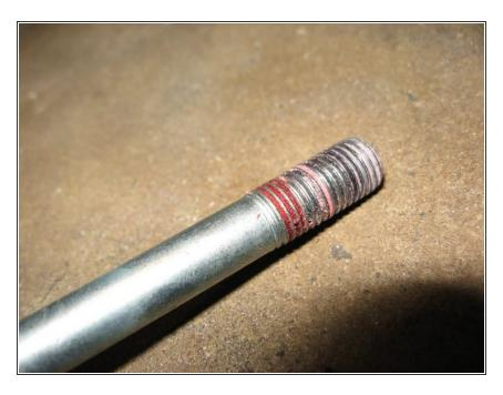
Bolt (silver one closer to the front of the block) with thread lock
