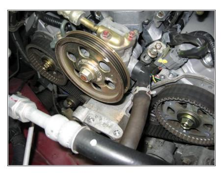
Upper and lower covers removed (12mm power steering adjuster nut shown)
