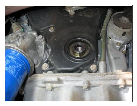
Lower cover showing crank end and lower part of the dipstick tube (hydraulic tensioner can be seen behind VTEC solenoid) (crank timing mark can also be seen)
