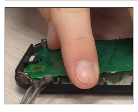
Remove keypad circuit board by lifting up circuit board while pulling clip.
