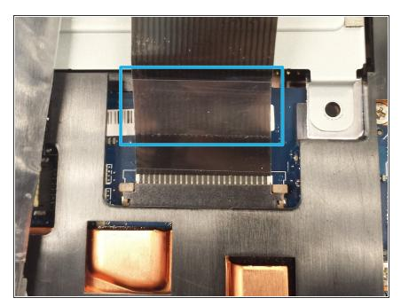
Pull the clear tab at the end of the ribbon towards the hard drive to detach the ribbon
