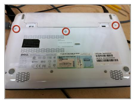
Using a Philip's head screwdriver, remove three screws: one directly below the battery and the other two to the right and the left of the two battery lock switches
