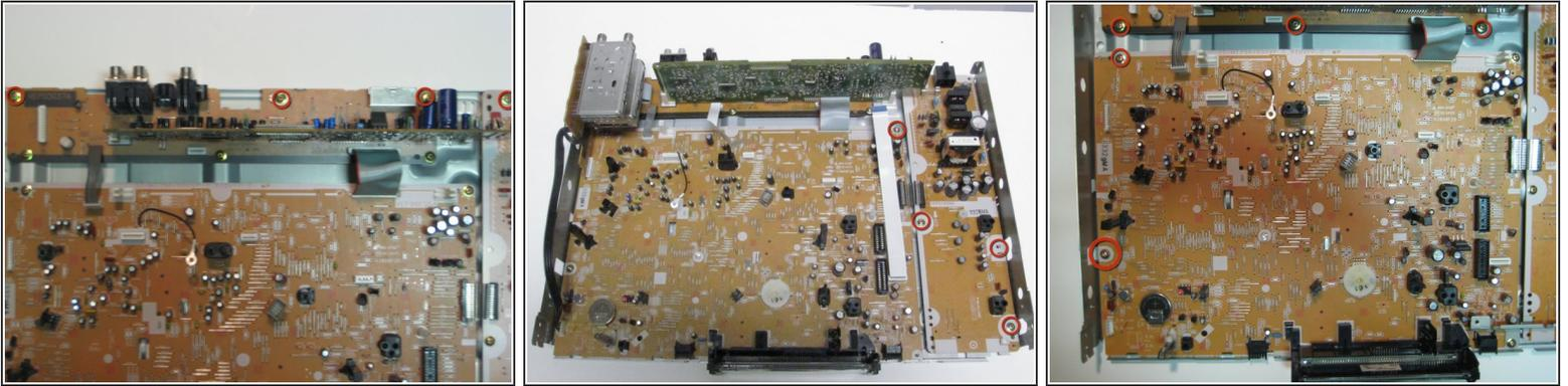
**⚠** Before replacing the motherboard, it is crucial to understand that this device cannot be taken apart any further without breaking solder points. So the motherboard, screen and power supply must be replaced together.
