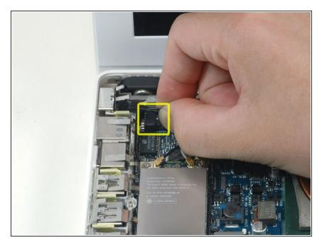
Disconnect the MagSafe board cable from the logic board.
