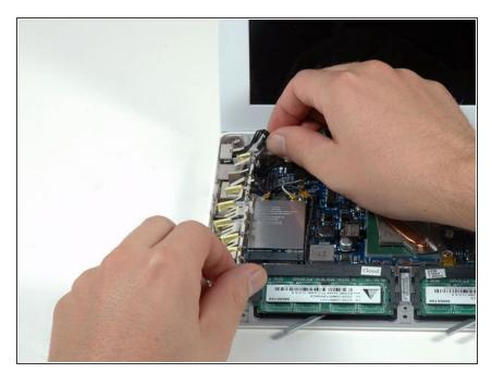
Lift the left I/O frame up and out of the computer. Pay attention to the thin metal EMI fingers, as they may catch as you remove the left I/O frame.
