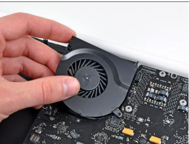
Removal of the fan was no biggie. It simply required a Phillips screwdriver and a spudger.
