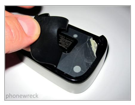
Peel back the Rubber pad on the bottom of the device.
