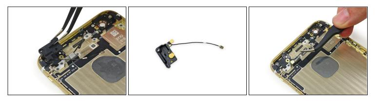
• We turn our focus to the top of the rear case enclosure, where a plethora of antennas await. These antennas prove to be no match for our trusty tweezers though.
