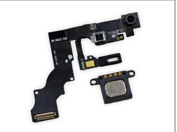
• The front-facing camera is part of a larger cable assembly, which includes the earpiece speaker, microphone, and ambient light sensor. Both reside on the front panel assembly.
