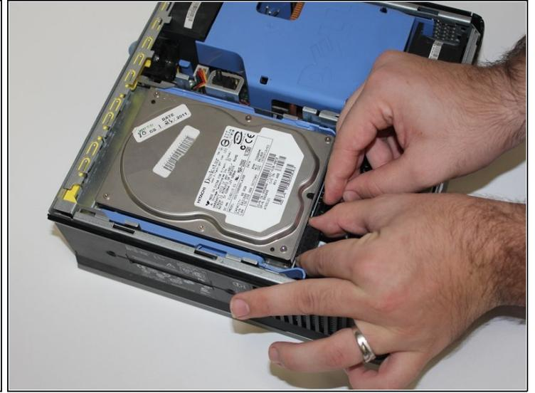
⚠ Ground yourself to avoid static from damaging any components. Either use a wrist strap and antistatic mat, or touch the metal computer case every few minutes.
