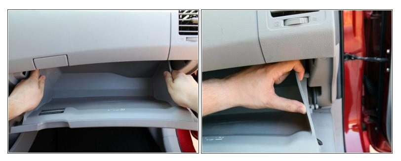
• Push the two side walls of the glovebox towards the center to free the stopper peg on each side.
