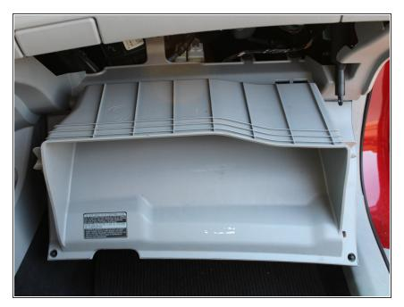
• Gently lower the glovebox to the floor. It should hang in the position shown.
