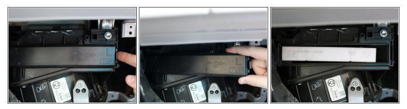
• Release the tab on the right side of the air filter cover, and swing it to the left. It should then easily pull away.
