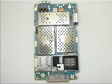
• Lift up from the top of the logic board as shown to remove.
