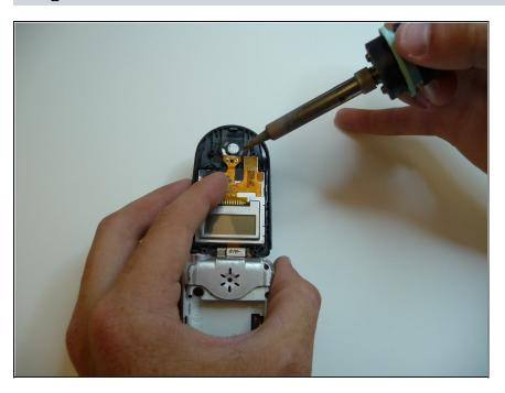
Use a soldering iron to detach the connector ribbon from the phone.
