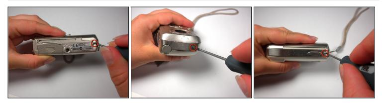
• Locate the 3 screws on the outer metal band and remove them with a #00 Phillips screwdriver.
