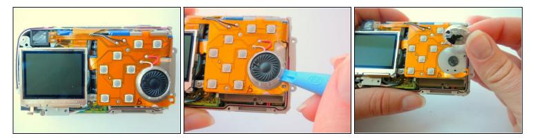
• Use a spudger to remove the speaker. It is attached by a double sided adhesive so it should just peel off.
