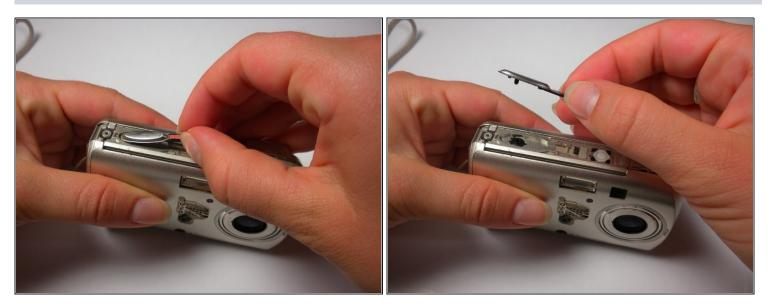
The shutter button can now be removed. It is not connected to the camera and can be lifted off.
