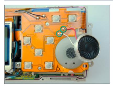
Un-solder the wires to remove the speaker.
