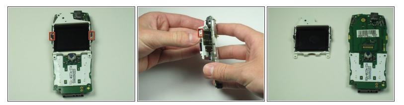
• Carefully remove the plastic clips holding the screen on the board.
