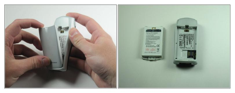
• Remove the battery from the back.
