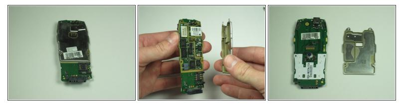
• Remove the plate protecting the more delicate processing parts from the logic board.
