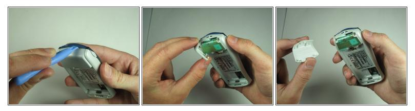
• Pry off the plastic cover from the top with a thin plastic shim, then remove it from the two bottom clips.
