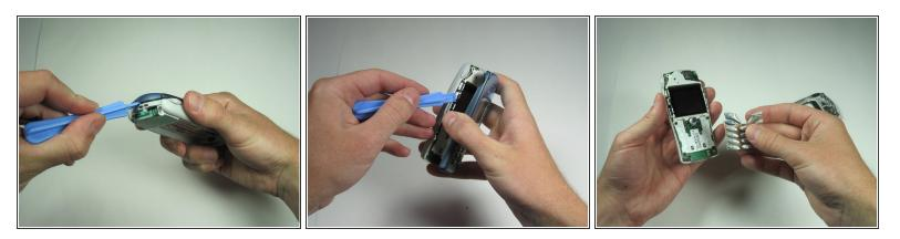
• After removing the screws, the two halves will separate. If not, then pry them gently apart.
