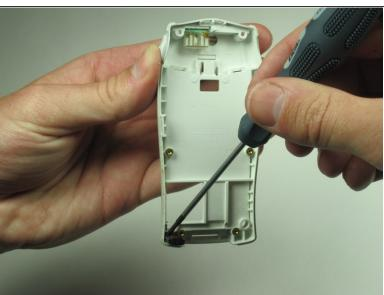
The microphone at the bottom of the rear housing can be levered out using a small screwdriver or any similar tool.
