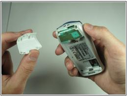
Pry off the plastic cover from the top with a thin plastic shim, then remove it from the two bottom clips.
