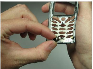
Remove the vibration motor visible in the front housing.
