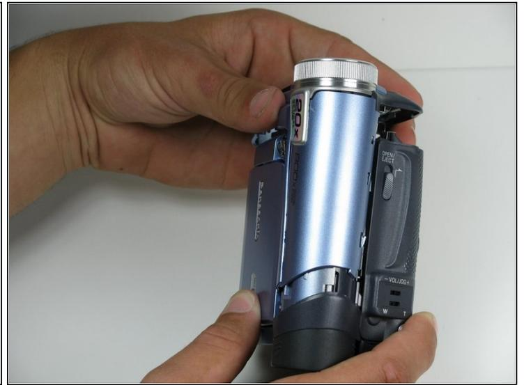
ⓘ Carefully remove the front cover from the body of the camcorder.
