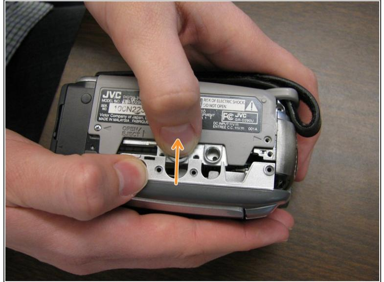
**⚠ Warning:** Avoid detaching the internal wiring by prying the camera apart slowly and carefully.
