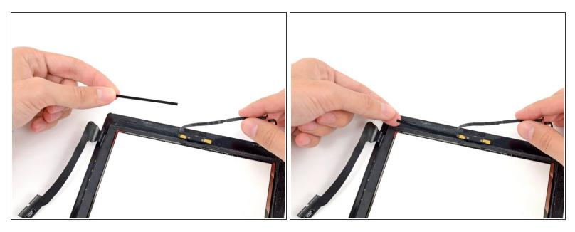
(i) It is recommened to lift the home button ribbon cable aside while placing the next adhesive strip.
