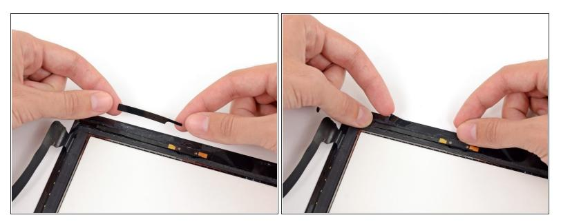
• Place the tabbed rectangular adhesive strip on the bottom right side of the front panel.
