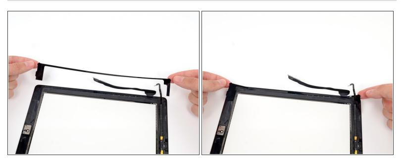
• Place the elongated **C** shaped adhesive strip on the right side of the front panel.
