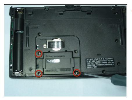
Using the same Phillips screwdriver, unscrew the remaining three 11.8mm screws.
