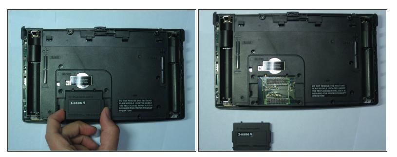
• Pull out the rectangular module when it is finally loose enough.
