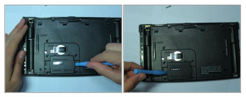
Using the Ipod Opening Tool pull up on both sides of the rectangular module while keeping the rest of the calculator flat on a surface face down
