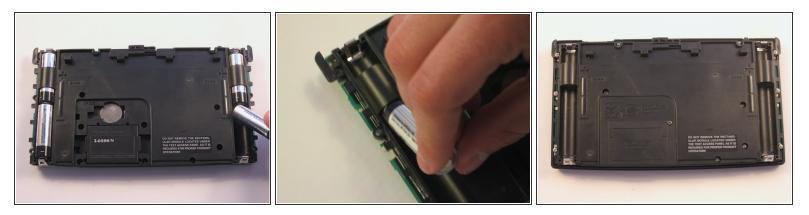
(i) The Batteries are now exposed and the calculator is face down with the back towards you.
