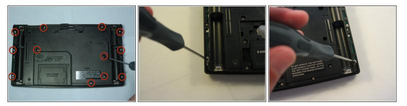
Using a Philips Screwdriver #00 unscrew the twelve 11.8mm screws shown in the picture and located on the back of the calculator.
