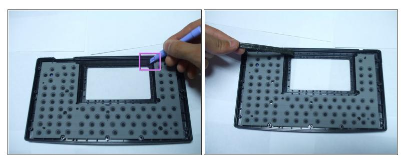
If one of the remaining strips is sticking to the others and can not be easily removed, use a tool such as the lpod Opening Tool to start pulling the strip up.
