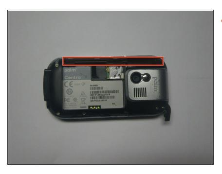
Remove the touchpad pen from the top left corner on the back to reveal the last of 6 screws to be removed.
