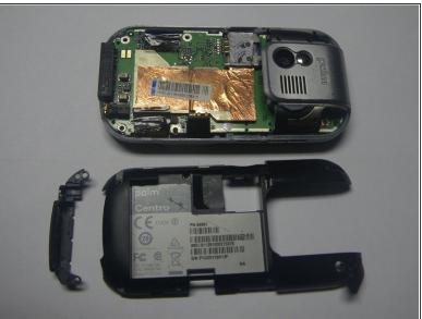
Continue with plastic pry tool all the way around the phone to remove the back housing.
