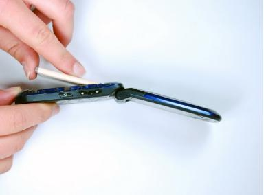
Simultaneously push the battery forward and pull up from the bottom.
