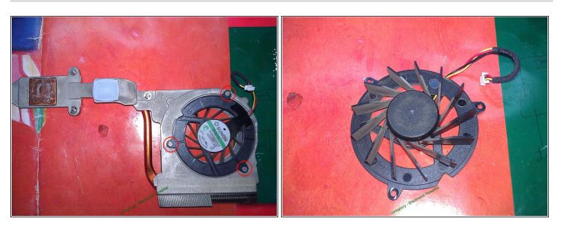
Remove these 3 screws to take the fan out of housing
