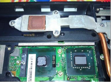
Apply new Thermal Glue and Thermal Pad to CPU and GPU chips. Be ready to reassemble the heat sink!
