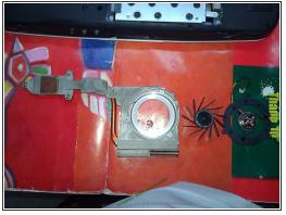
Now we clean the housing. Remove the dust stuck inside and outside ventilation leaves by a brush. Using a high pressure pump to clean is much better in this situation
