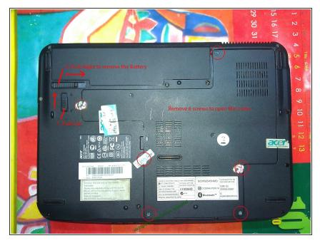
Now, turn the laptop upside-down. We push 2 buttons to take out the battery. Then remove 6 screws to open the cover as shown in the picture
