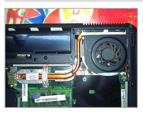
There are 4 screws numbered from 1 to 4. We should remove them in order of sequence, from 1 to 4. Use screwdriver to twist anticlockwise
