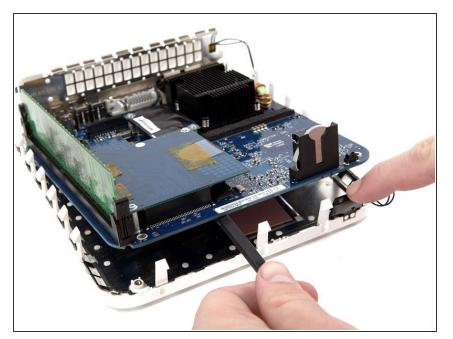
Use one hand to slide a spudger underneath the logic board and the other to pull back on the black sleep light unit. Lift up the with the spudger to free the logic board from the lower case and use both hands to slide the logic board toward you.
