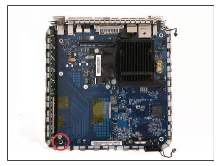
Remove the single black Phillips screw from the front left corner of the logic board.
