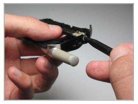
On the back casing, using a spudger, push into the headphone jack at an upward angle to pop it out
