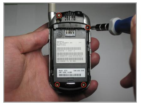
Using a Hex T6 screwdriver, remove the 4 screws holding the back plate of the phone in place
