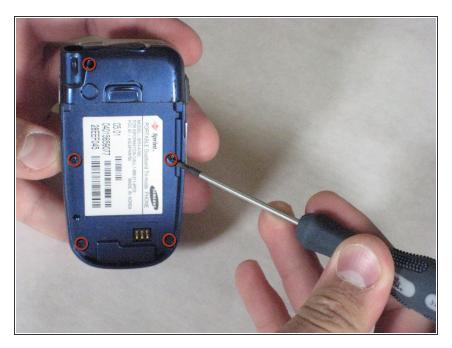
• Remove the five screws as shown.
