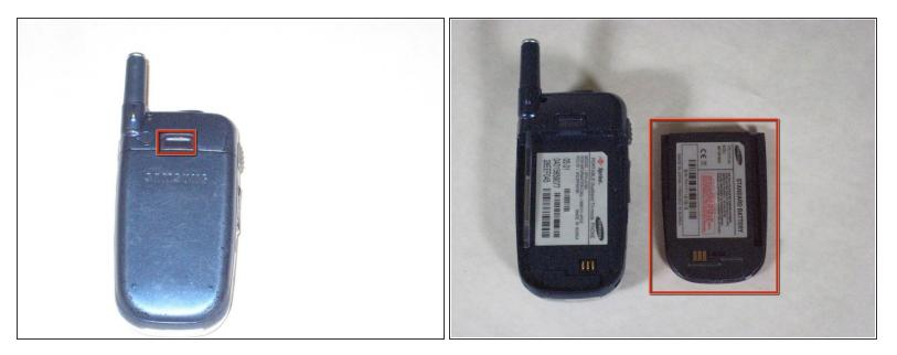
• Push open the latch and remove the battery.
